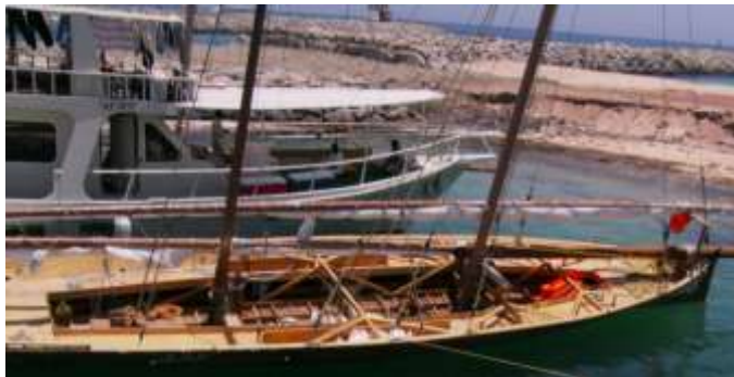
Forty-foot dhow, lightly built & strongly braced for racing Photo: Michael Creamer
