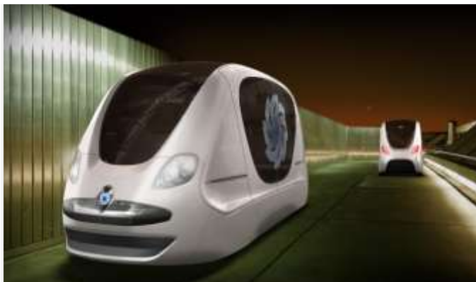
PRT - Personal Rapid Transport system pod A key component of the multi-layered system at Masdar
